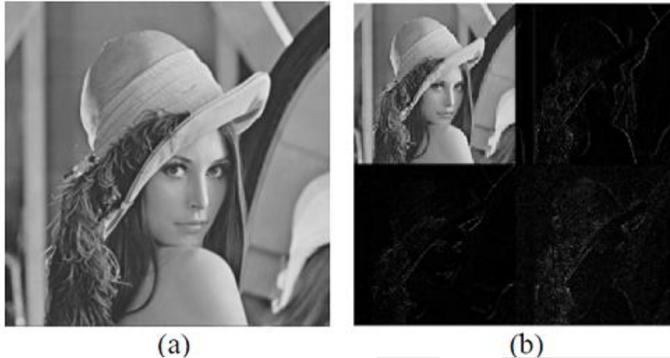
Figure 3. (a)Original image-Lena, (b) Result after the first-order 2-D Haar-DWT
