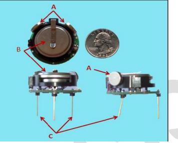
Figure 3. A prototype Kilobot module (top view in upper left, front view in lower left, side view in lower right) next to a US quarter for scale. Some features are (A) vibration motors, (B) battery, (C) slanted legs.
