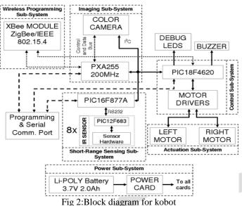
The overall system design of Kobot is shown in Figure 2. At the heart of the Kobot, there is the control sub-system to which all of the information from the other sub-systems, that is short range sensing, communication, vision and power, are fed to the control sub-system. With the information acquired, a 20MHz PIC16F877A, called the main controller, implements the control algorithm which determines the behaviors of Kobot.
