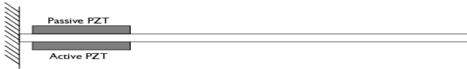
Figure 5: A piezoelectric actuator with an active piezoelectric device below and a passive piezoelectric device above the silicon bar.
