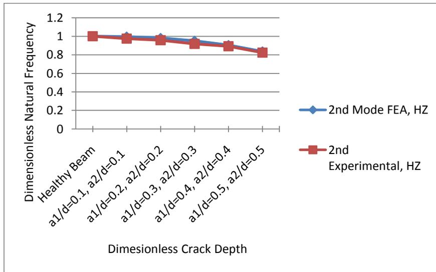
Fig.9 Comparison of FEA and Experimental Modal Analysis Results for 2<sup>nd</sup> mode of vibration
