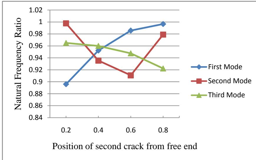
Fig.16 Natural frequency ratio at different crack positions for  $L_1=0.25$ ,  $a_1=0.2$  and  $a_2=0.2$
