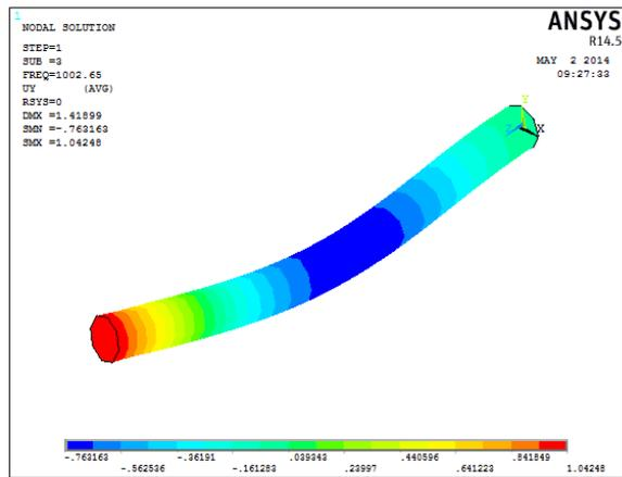
Fig.3 2<sup>nd</sup> Mode of Vibration (Healthy beam)
