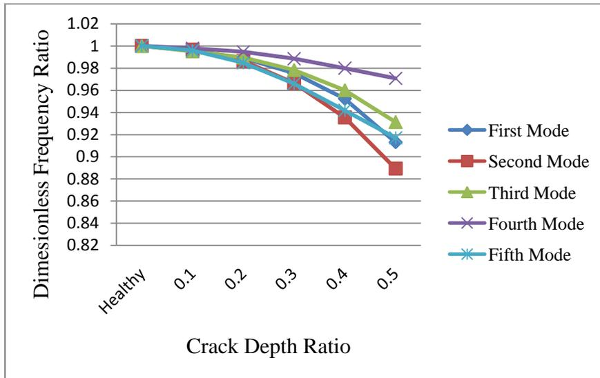
Fig.12 Natural Frequency ratio at different crack depths for  $e_1=0.3$  and  $e_2=0.4$
