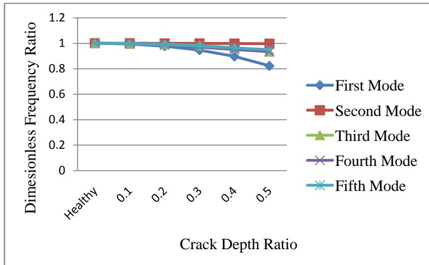
Fig.11 Natural Frequency ratio at different crack depths for  $e_1=0.3$  and  $e_2=0.2$
