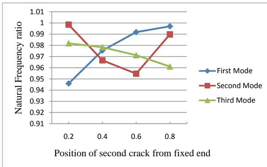
Fig.17 Natural frequency ratio at different crack positions for  $L_1=0.25$ ,  $a_1=0.3$  and  $a_2=0.3$
