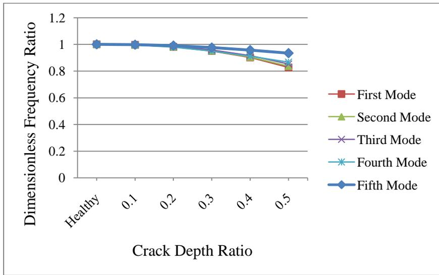
Fig.10 Natural Frequency ratio at different crack depths for  $e_1=0.25$  and  $e_2=0.55$
