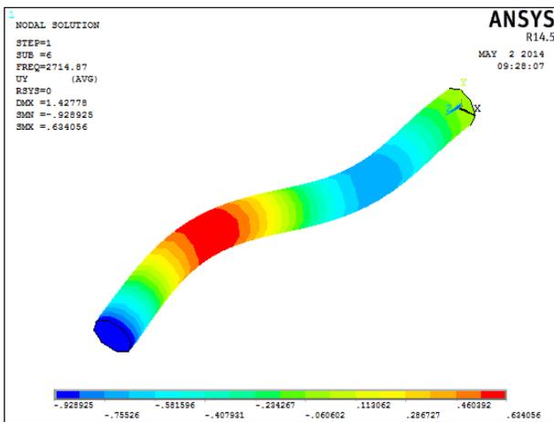
Fig.4 3<sup>rd</sup> Mode of Vibration (Healthy beam)
