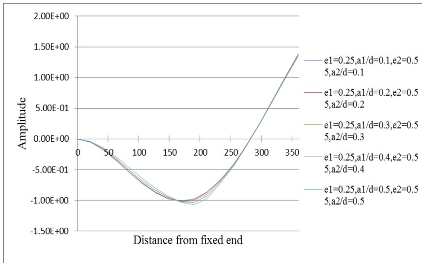
Fig.19 Mode shapes of 2<sup>nd</sup> mode of vibration
