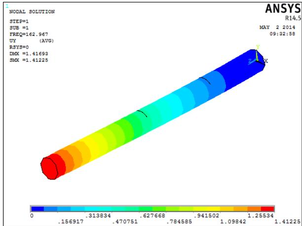
Fig.5 1<sup>st</sup> Mode ( $e_1=0.25, a_1/d=0.1, e_2=0.55, a_2/d=0.1$ )
