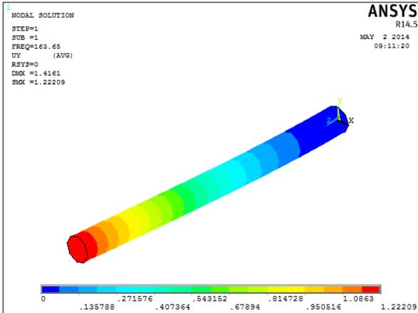
Fig.2 1<sup>st</sup> Mode of Vibration (Healthy beam)
