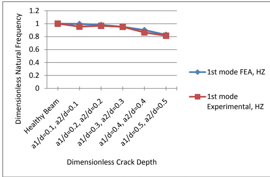
Fig.8 Comparison of FEA and Experimental Modal Analysis Results for 1<sup>st</sup> mode of vibration
