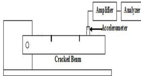
Fig. 1 Test rig for Experimental Modal Analysis
