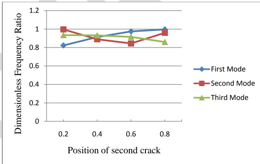
Fig.15 Natural frequency ratio at different crack positions for  $L_1=0.25$ ,  $a_1=0.1$  and  $a_2=0.1$
