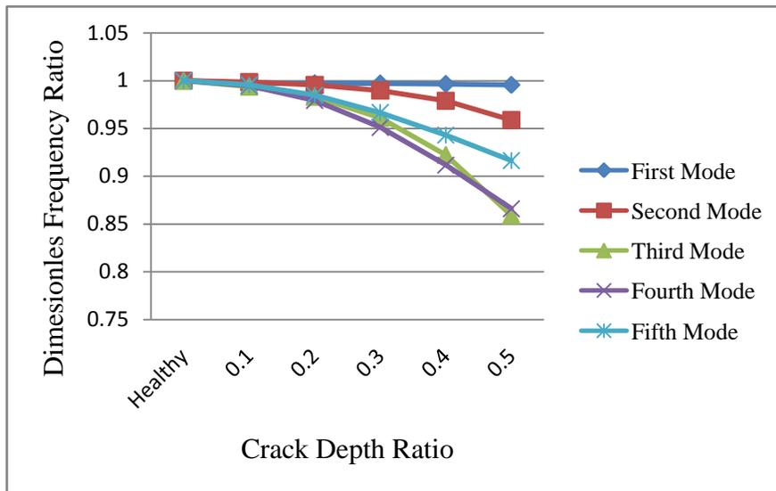
Fig.14 Natural Frequency ratio at different crack depths for  $e_1=0.3$  and  $e_2=0.8$
