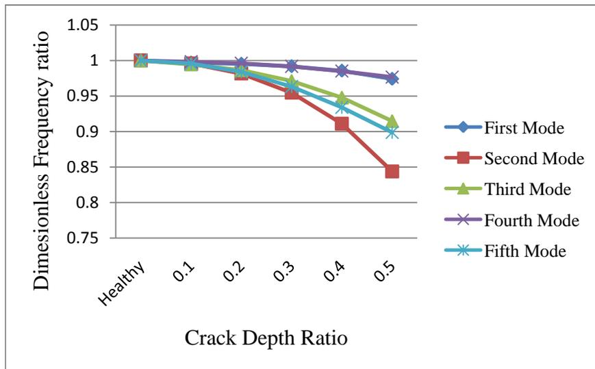
Fig.13 Natural Frequency ratio at different crack depths for  $e_1=0.3$  and  $e_2=0.6$
