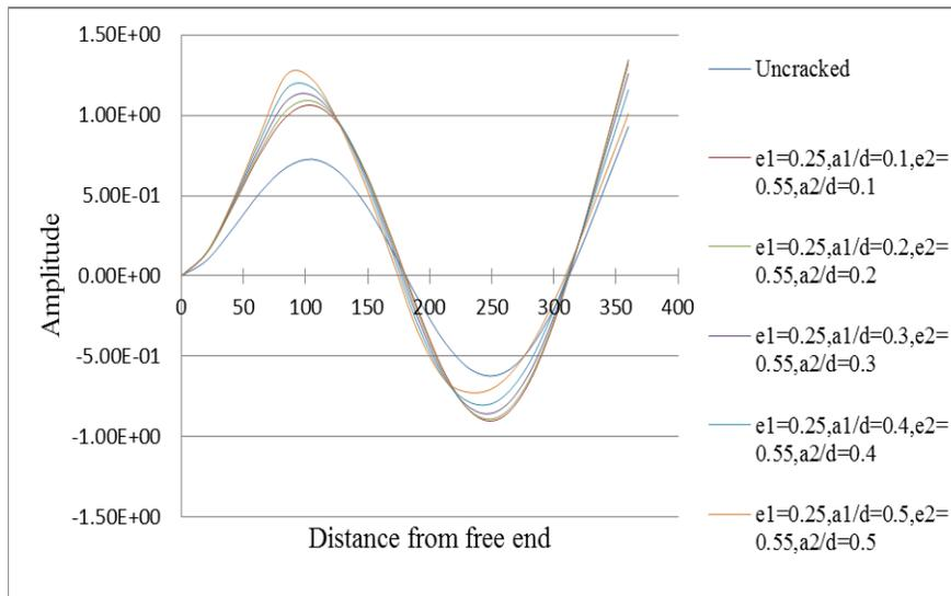
Fig.20 Mode shapes of 3<sup>rd</sup> mode of vibration
