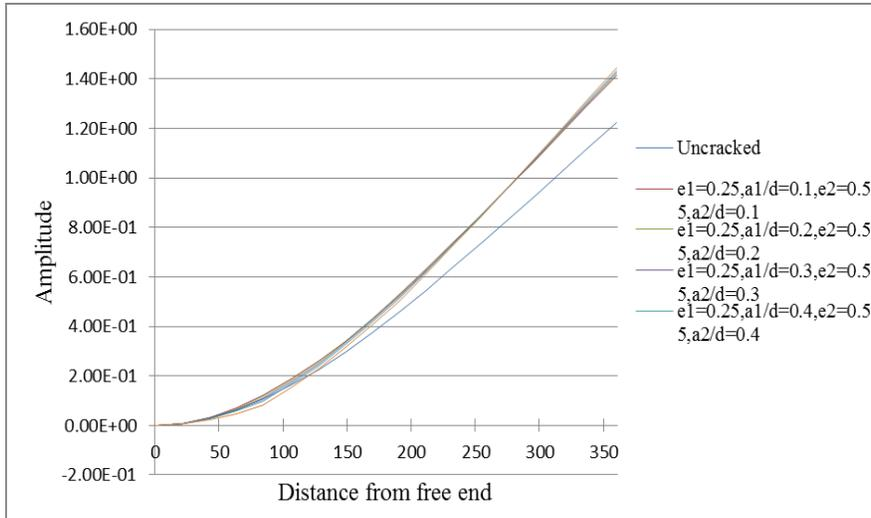
Fig.18 Mode shapes of 1<sup>st</sup> mode of vibration
