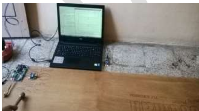
Figure 8: Experimental setup for vibrations given at less than 1 foot
