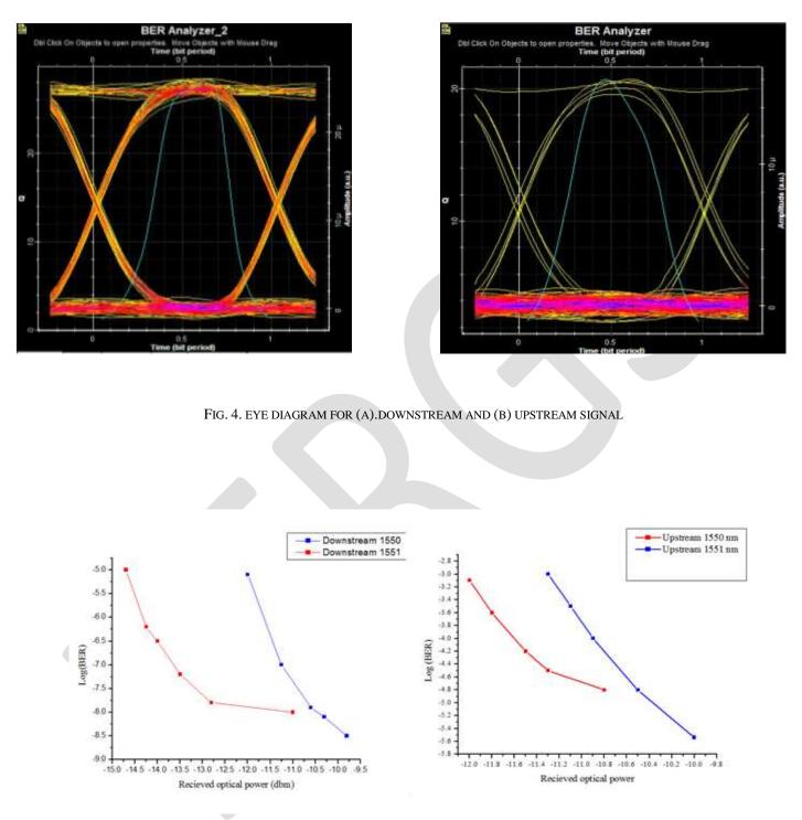
Fig. 5.Transmission performance of downstream and Upstream data
