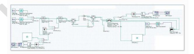
Fig 3 : Simulation Block of architecture with sech pulse generator
