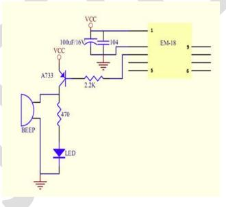
Fig4: EM-18 Application Circuit
