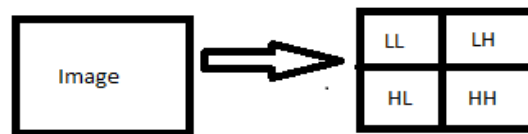
Fig. 5. One filter stage in 2-D DWT
