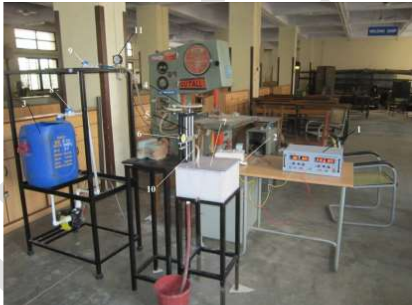
1.DC power supply, 2.feed control circuit, 3.electrolyte tank, 4.gear train, 5.linear vertical slide, 6.dial gauge, 7.machining chamber, 8.bypass valve, 9.flow control valve, 10.tool holder, 11.pressure gauge
