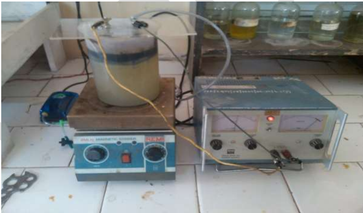
Figure No 4. Experimental setup of Electro Coagulation Process with aeration
