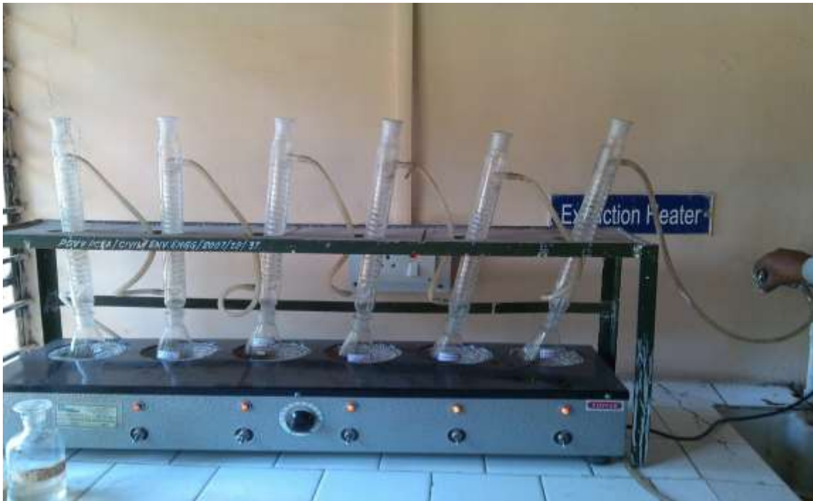
Figure No 2. COD Hot Plate with Temperature Regulator
