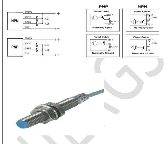
PNP Normally Open: provides voltage to BR & BL, the resistor such as 1K can be used as a load. BK will provide a positive voltage if the metal object presence. Therefore, you can use BK & BL to power a motor or a light when the metal part is presence.
