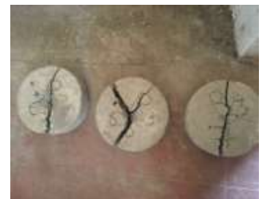
Failure pattern for R3
