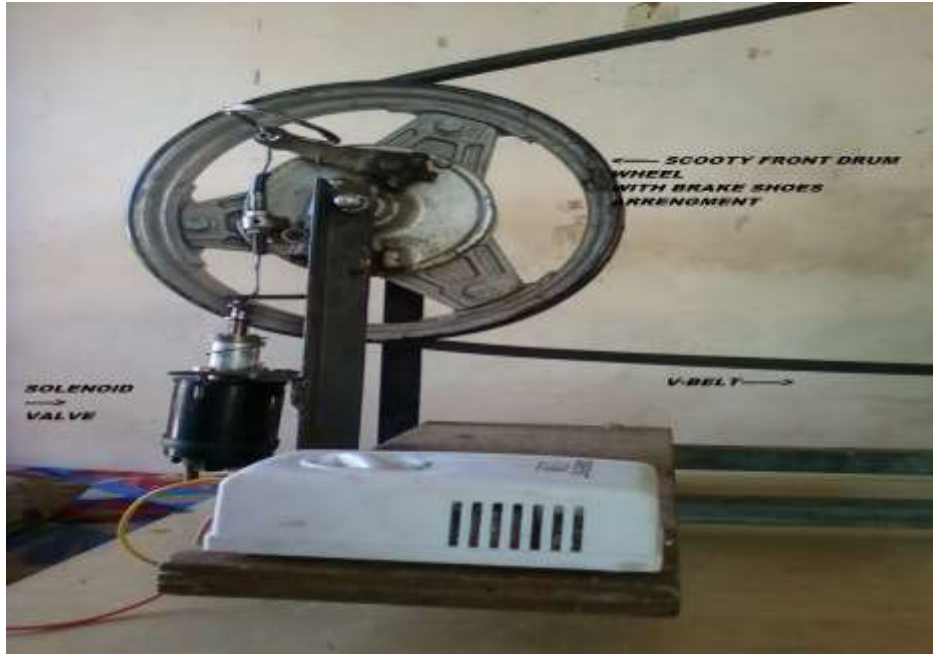
Figure 12. Wheel attaches with valve and brake drum
