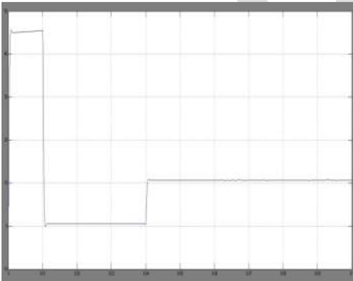
Fig. 14 Current at load applied at t=0.04\text{sec}
