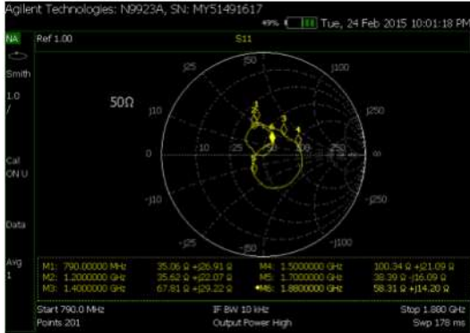
Figure 7. Smith CHART of the Antenna
