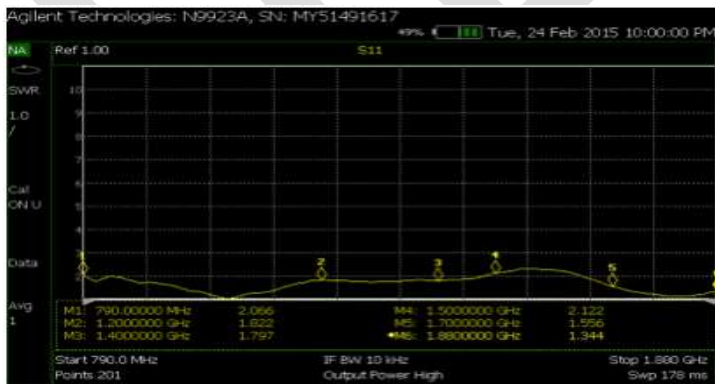
Figure 6. VSWR of the Antenna
