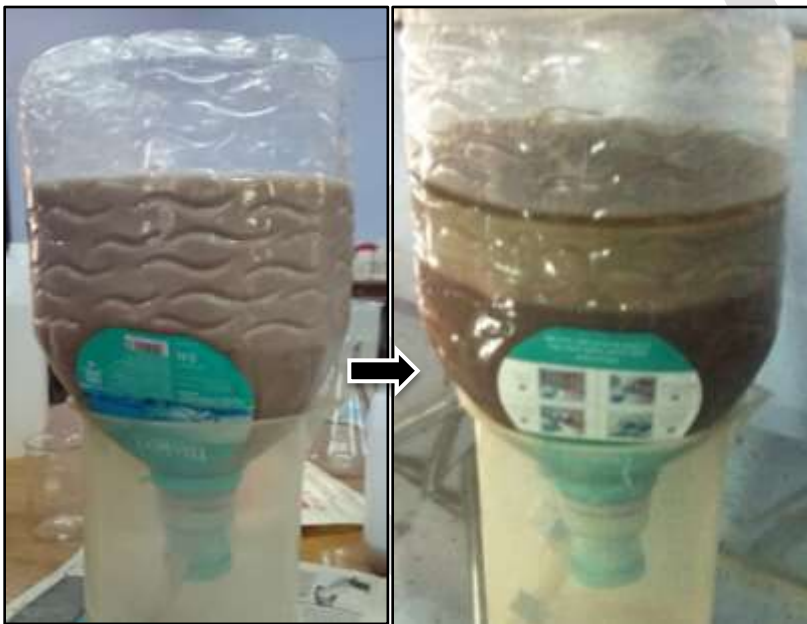
Fig. 2: Formation of Sludge post 24- 48 hrs standing time
