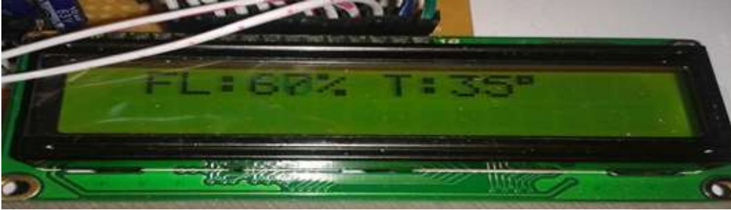
Fig. Result of fuel level and temperature sensor in percentage indicated on LCD
