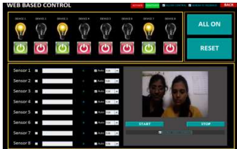
Fig 5: Environment for Device Control ,sensors values, Video Feedback
