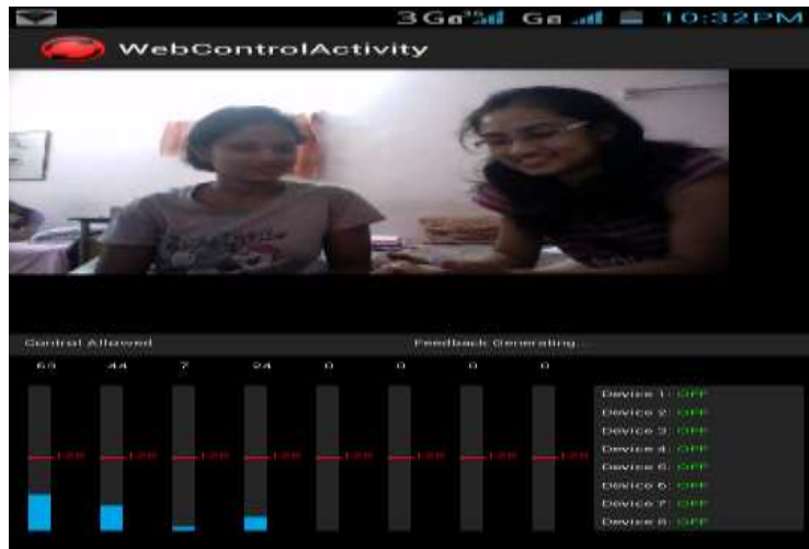
Fig 7 : Environment to see the Video Feedback,Device Status and Sensors Value in Android App
