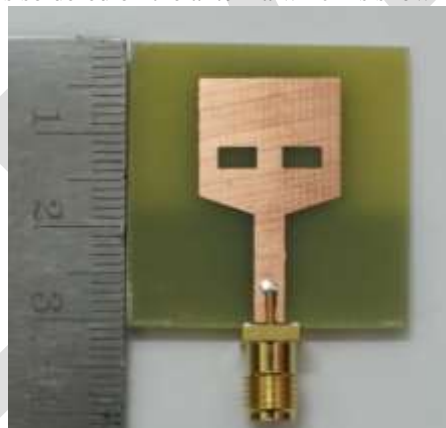
Figure 8. Fabricate Antenna (Top View)
