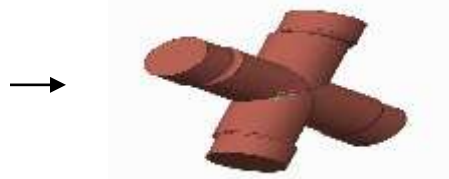
Figure 2 Shearing Failure In Existing Pin Of A Universal Coupling
