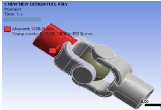
Figure 19 Moment Applied To Proposed Assembly
