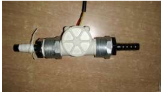
Fig 2: Flow rate meter
