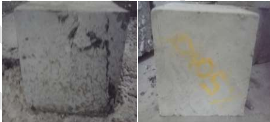
Fig.4.1 Cube failure pattern in M30 plain concrete and Kektad fiber reinforced concrete with 0.05% F-C ratio (28 days curing)
