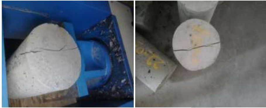
Fig.4.2 Cylinder failure pattern in M30 plain concrete and Kektad fiber reinforced concrete with 0.05% F-C ratio (28 days curing)
