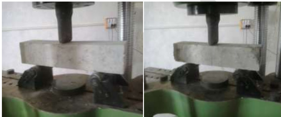
Fig.4.3 Flexural failure pattern in M30 plain concrete and Kektad fiber reinforced concrete with 0.05% F-C ratio (28 days curing)
