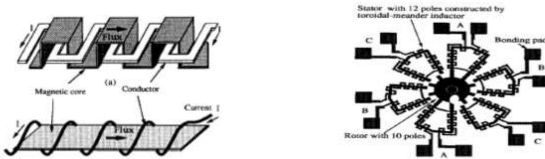
Fig.1 Electromagnetic induction micromotors basic structure and operation [1, 2]
