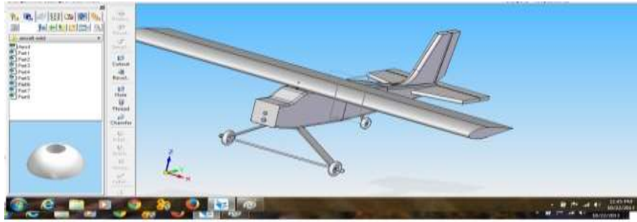
Fig 15: Final Completed view of our High Winger, Conventional tail aircraft in Solid Edge.
