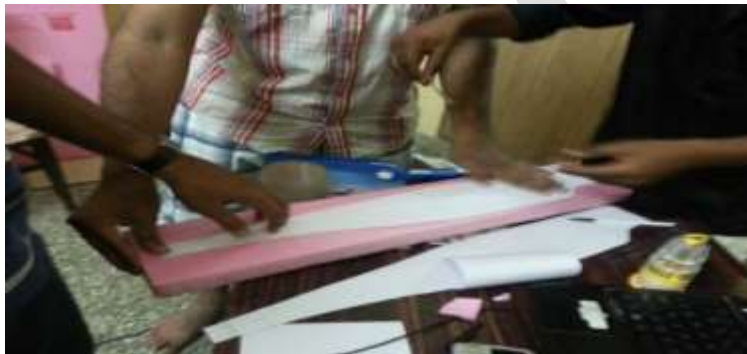
Fig 27: Sticking the 2D draft of the fuselage on to the Styrofoam material.
