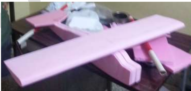
Fig 33: View after cutting & sanding of the Styrofoam material.
