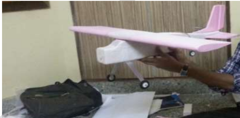
Fig 35: Assembly of the Wing & Landing gears to the fuselage.
