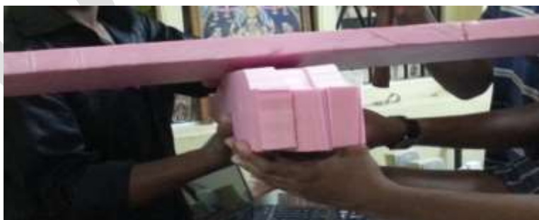
Fig 29: Styrofoam material cut in layers so as to form the fuselage.
