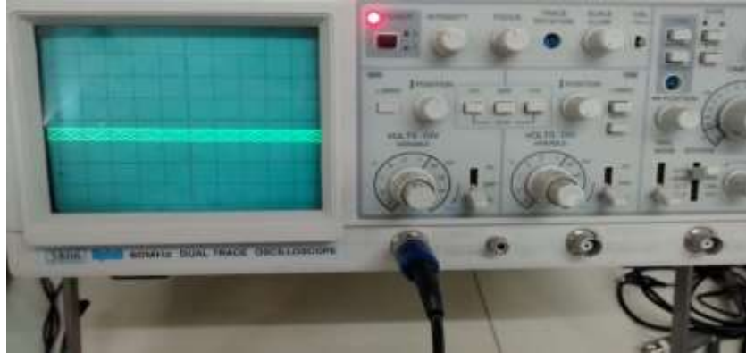
Fig 4.8 Output for fixed gain DAC code 1536 and varying bias DAC code 1024
