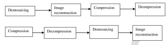
Figure 2 a) Demosaicing first scheme b) compression first scheme
