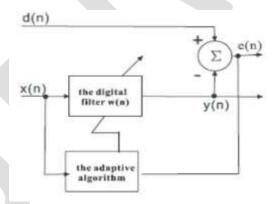
Figure 1: Adaptive filter scheme
