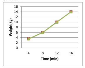
The above graph shows Time V/s kilogram. The graph clearly shows that the amount of pieces collected with respect to time. In this test 5 feet length and 4 coconut leaves are taken. The test is conducted for 4 different times. For which results are obtained, how much amount of powder collected and graph is plotted.
