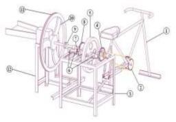
Fig1: Pedal operated shredder machine
