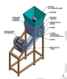
Fig4: Coconut leaves shredder.
