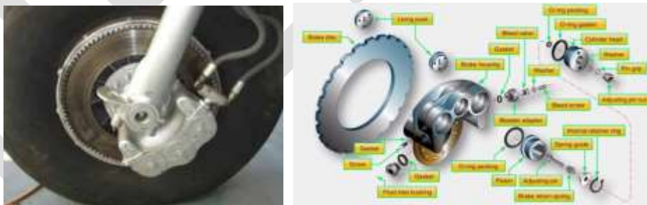
Fig 1: Aircraft disc brake and exploded view
