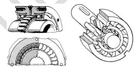
Fig.1.Frictional free-play mechanism
