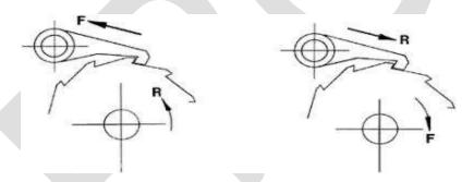
Figure 3: Variation of ratchet and pawl action (F =force; R = reaction).
