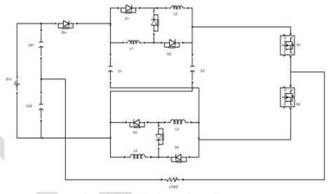
Figure. 2: Switched Inductor Z Source Converter The proposed converter performs differently in two cases: $D_1 + D_2 \le 1$  and  $D_1 + D_2 > 1$ .
