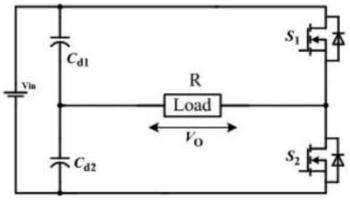
Figure.1 : Conventional half-bridge converter
