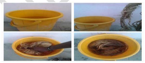
Fig. 1 Kenaf fiber is treated with NaoH solution for 24hrs to remove impurities and increase the strength of the fiber
