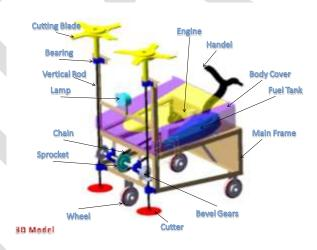
Fig 4: 3D Model of Sugarcane Harvesting Machine
