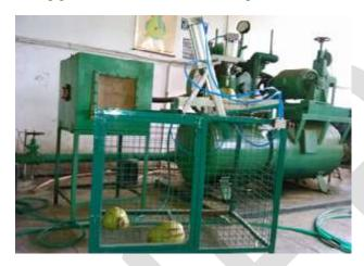
Fig 5 : Working model of punch cum splitter for tender coconut
