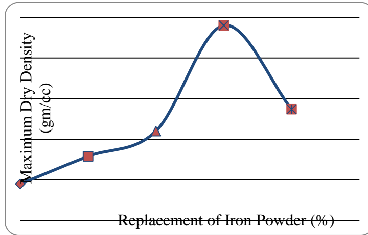
Figure 4: Variation of Maximum Dry Density with replacement of Iron Powder
