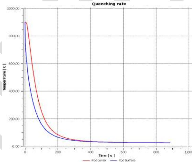
Fig: Temperature Vs Time for 60% concentration by mass of ethylene glycol
