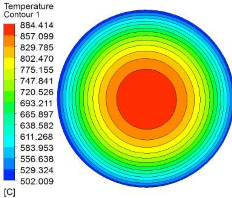
Fig: Horizontal temperature plot after 10 sec during trial when ethylene glycol concentration is 40%.
