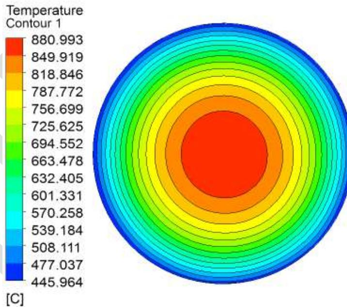
Fig: Horizontal temperature plot after 10 sec during trial when ethylene glycol concentration is 20%.
