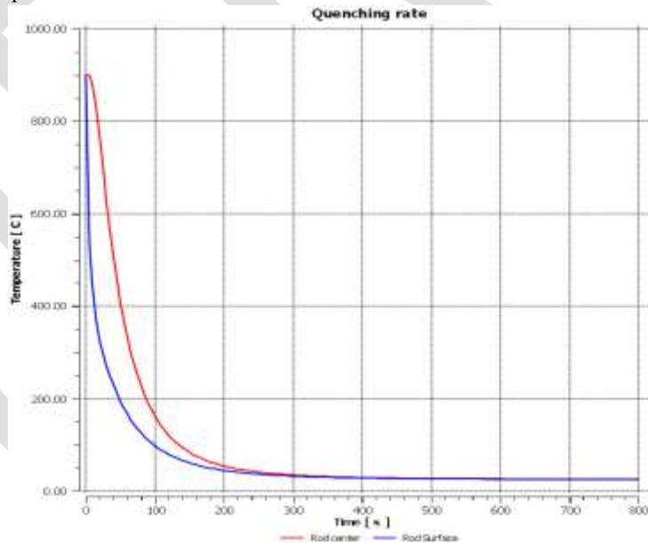
Fig: Temperature Vs Time for 20% concentration by mass of ethylene glycol
