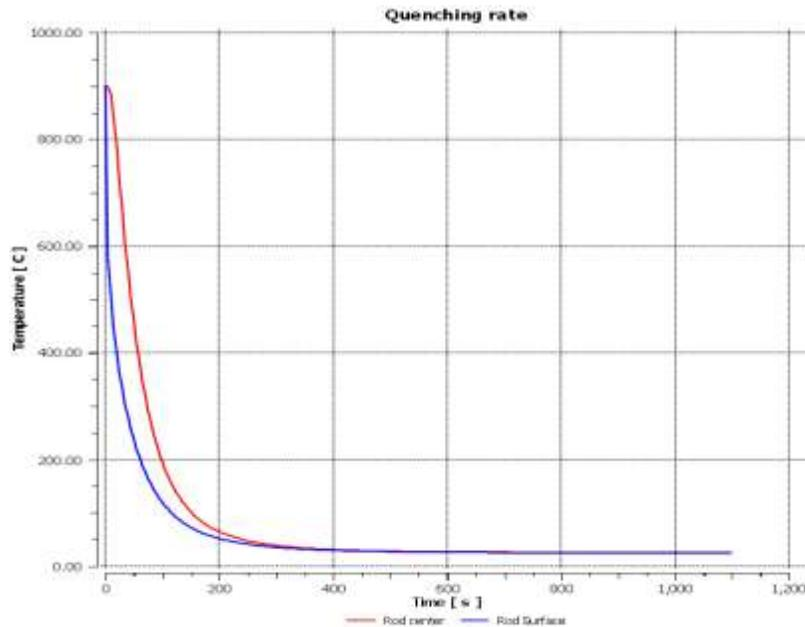
Fig: Temperature Vs Time for 40% concentration by mass of ethylene glycol
