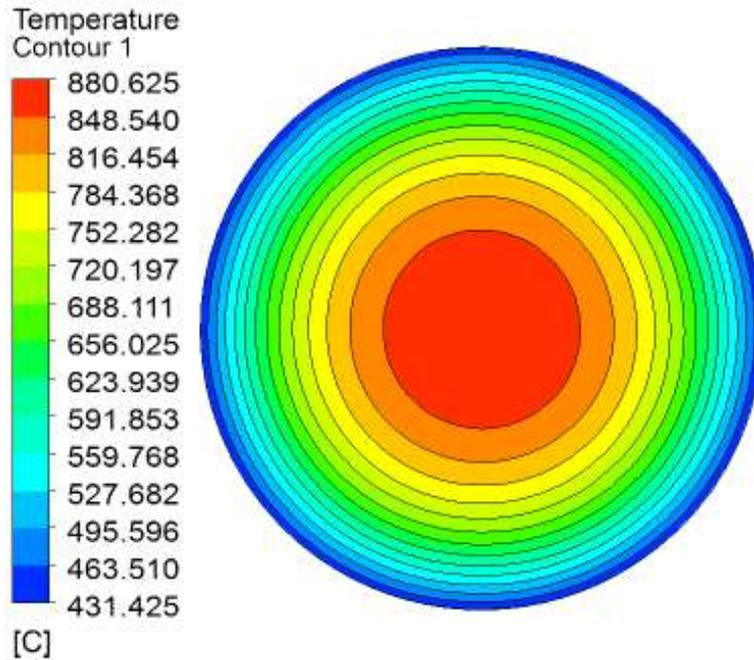
Fig: Horizontal temperature plot after 10 sec during trial when ethylene glycol concentration is 0%.
