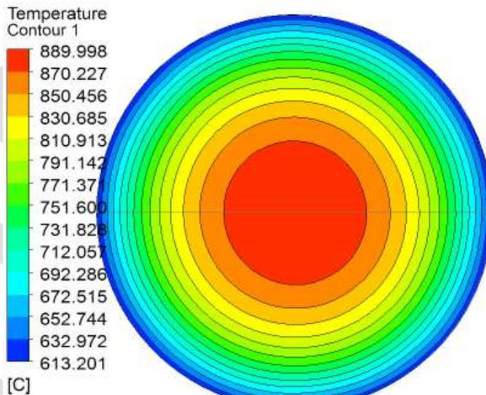
Fig: Horizontal temperature plot after 10 sec during trial when ethylene glycol concentration is 60%.
