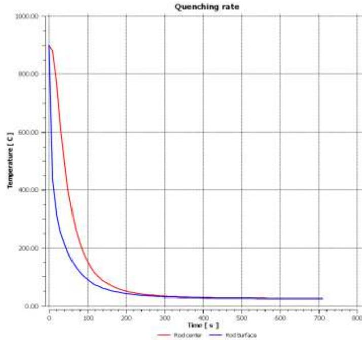
Fig: Temperature Vs Time for 0% concentration by mass of ethylene glycol
