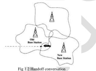
When a MS moves away from its current AP, it must be reconnected to a new one to continue its operation. The search for a new AP or base station (BS) and following registration without any loss is known as handover and the time required to complete a handover process is known as handover latency. Figure 1.2.1 shows the scenario of horizontal and vertical handover.
