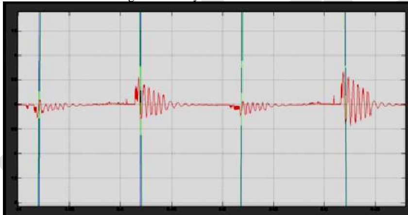
fig. 16 Common mode leakage current
