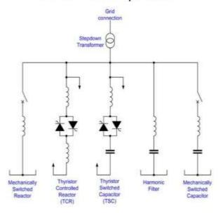
Fig. 1. Static VAR Compensators
