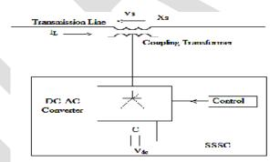
Fig.3. Static synchronous series capacitor
