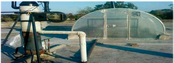
Fig.4 Solar Biomass Hybrid Drying System
