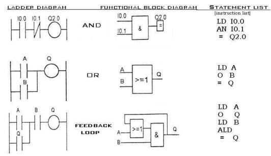
Figure 2. Comparison between PLC program logics
