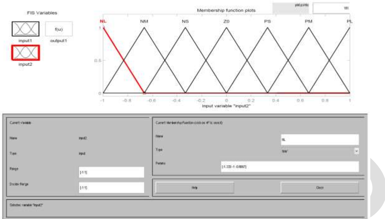
Fig.4. Membership function of the input error ( e ).
