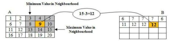
Figure(2): Range filtering function
