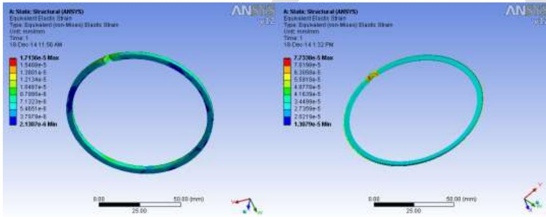
FIGURE 8.4 STRAIN IN COATED PISTON RINGS
