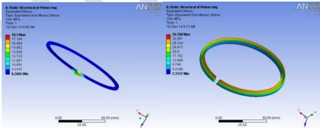
FIGURE 8.5 STRESS ACTING ON UNCOATED PISTON RING
