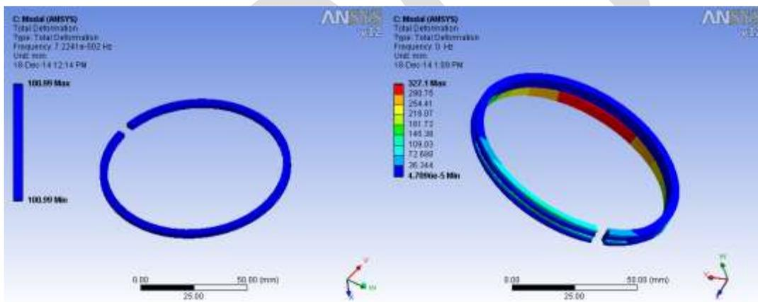
FIGURE 8.10 TOTAL DEFORMATION IN COATED PISTON RINGS
