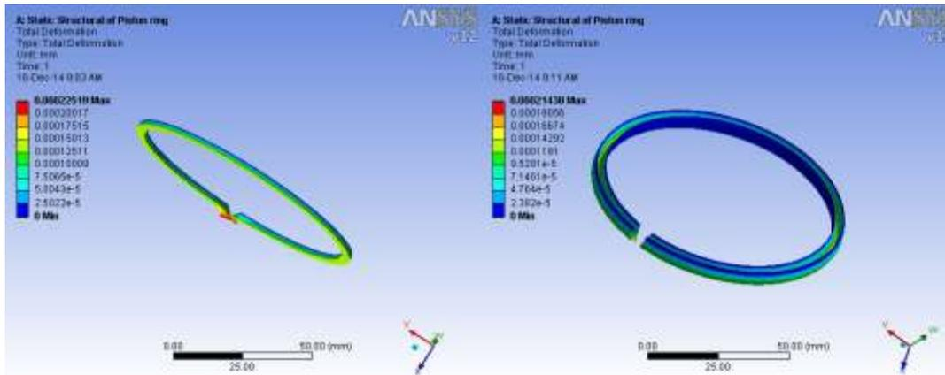
FIGURE 8.1 TOTAL DEFORMATION OF UNCOATED PISTON RINGS
