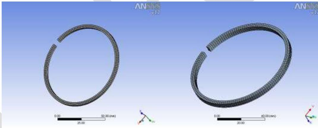
FIGURE 7.2 MESHED MODEL OF PISTON RING PACK
