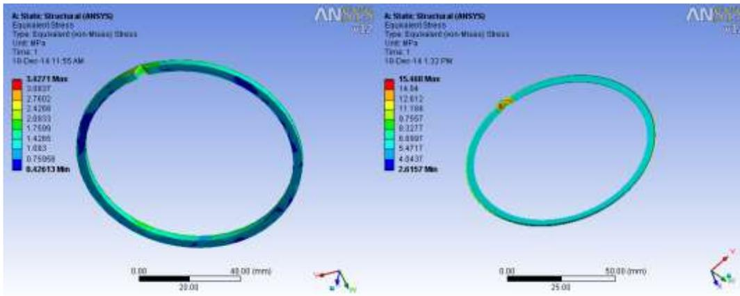
FIGURE 8.5 STRESS ACTING ON COATED PISTON RINGS
