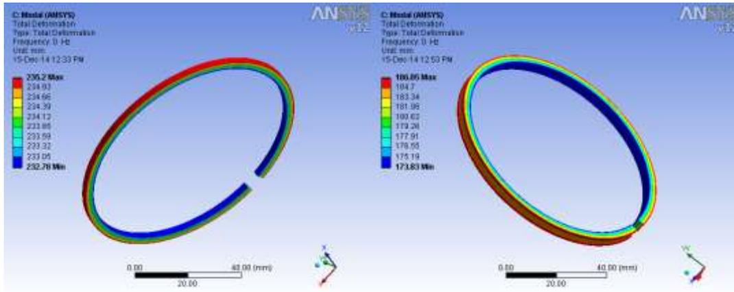
FIGURE 8.9 TOTAL DEFORMATION IN UNCOATED PISTON RINGS
