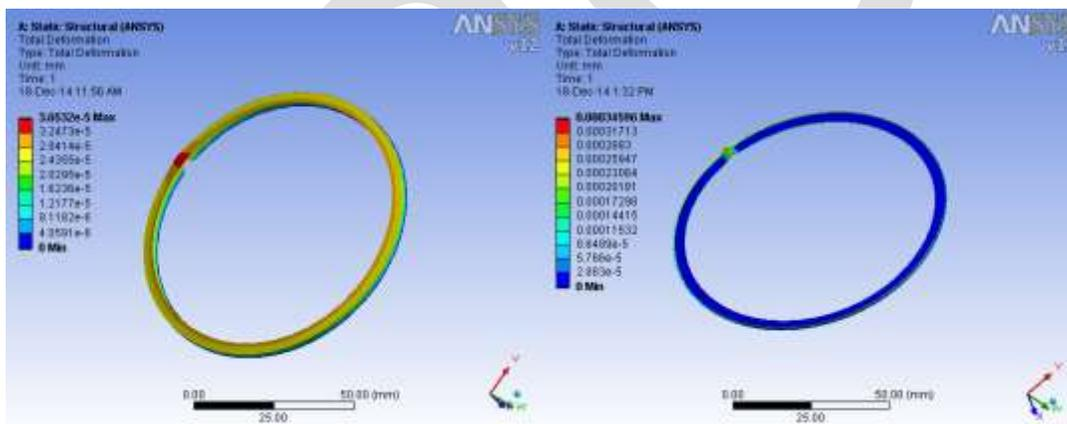
FIGURE 8.2 TOTAL DEFORMATION OF COATED PISTON RINGS
