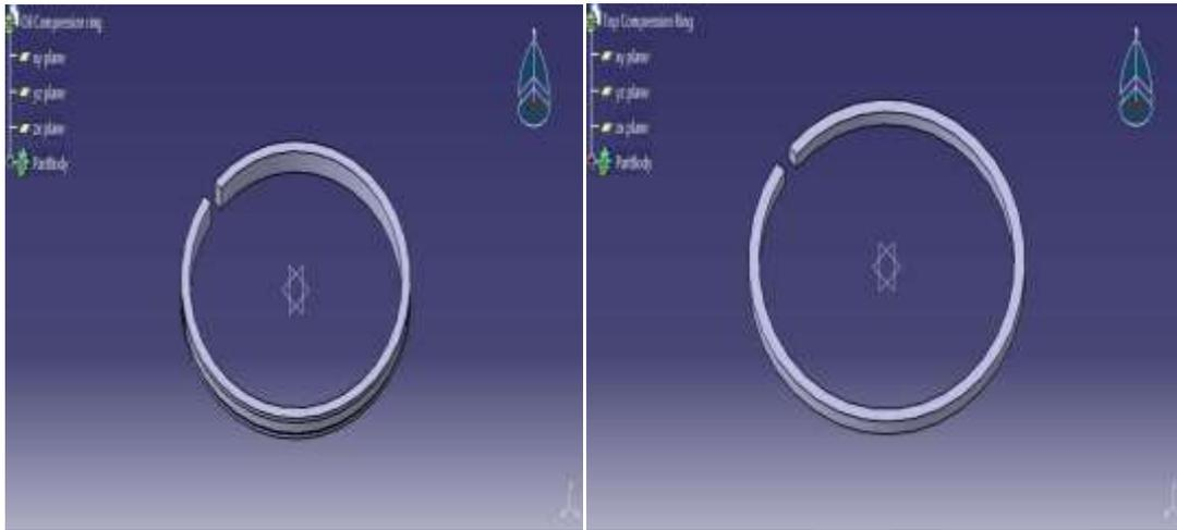
FIGURE 7.1 GEOMETRY MODEL OF PISTON RING PACK
