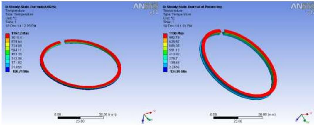
FIGURE 8.6 TEMPERATURE DISTRIBUTION OF COATED PISTON RINGS
