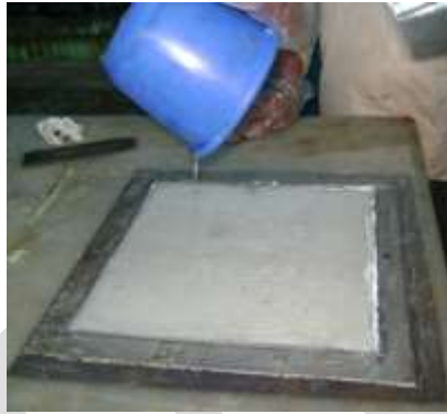
Fig -2: Pouring of Epoxy Resin
