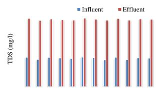
Number of Batch experiments Figure 5.Impact of struvite precipitation on the concentration of TDS of dairy wastewater
