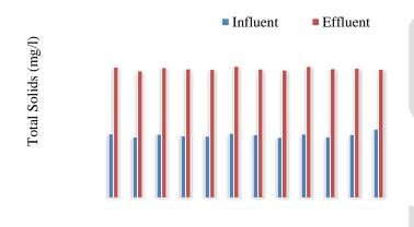
Number of Batch experiments Figure 6.Impact of struvite precipitation on the concentration of TS of dairy wastewater
