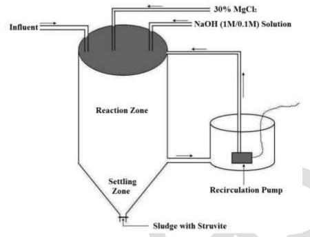
Figure 1. Schematic sketch of Struvite Fed Batch Reactor
