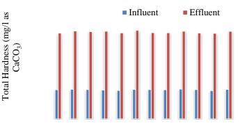
Number of Batch experiments Figure 9. Impact of struvite precipitation on the concentration of Total Hardness of dairy wastewater
