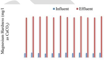
Number of Batch experiments Figure 11. Impact of struvite precipitation on the concentration of Magnesium Hardness of dairy wastewater
