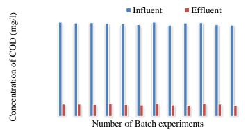
Figure 8. Impact of struvite precipitation on the concentration of COD of dairy wastewater
