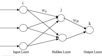
Fig. 2: Typical Neural Network Computational Structure
