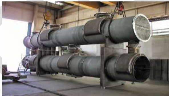
Stacked Heat Exchanger
