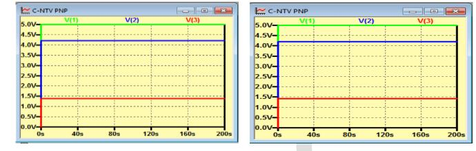
Figure 6: VIN (V1) = 5v NTV V (3) = 1.37V R1= 125Ohms. Figure 7: VIN (V1) = 5v NTV V (3) = 1.37V R1= 10KOhms.
