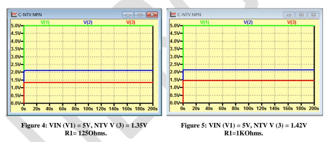
So the power can be easily calculated for different input voltages and power ratio can be determined. That is, the Power Ratio = 200 mW/15.015 mW = 13.32. So the power reduction is almost 13.32 times which can easily be carried out in large CMOS IC's. The simulated results show that for large current load at 1250 hms the output is 1.35V and for small current load at 1K0 hms the output is 1.42V. So the regulation of NTV has the reliability of more than 95%.
