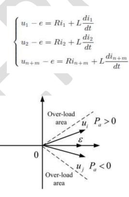
Fig. 5 Output power control by phase adjustment.
