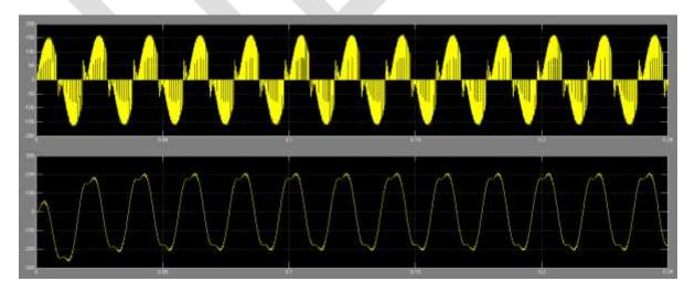
Fig.11 Output voltage and current at load (induction motor).
