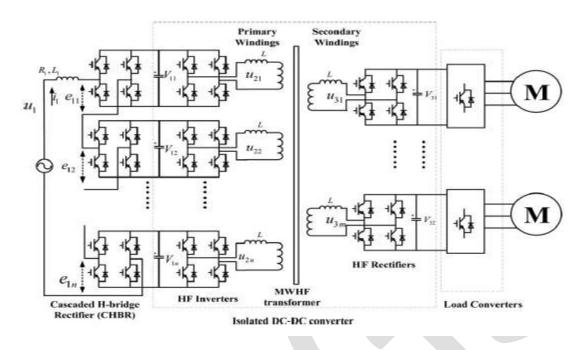
Fig. 1 General topology of proposed converter
